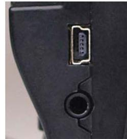
If you wish to charge the Telemetry-Box "on the road", use a USB adapter for your car's cigarette lighter; USB adapters for domestic use are also available. Use only a USB charger rated at 5 V / 1 A.
