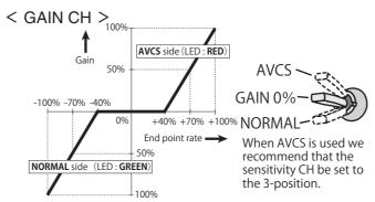
Refer to the transmitter instruction manual and set the end point. When AVCS is used, setting the 3-positions switch to the sensitivity CH (there are types which cannot be set by transmitter) and setting it as shown above is recommended. In the case of a 2-positions switch, inhibiting the gyro at 0% sensitivity such as NORMAL mode and sensitivity 0% and AVCS mode and 0% sensitivity is safe.
