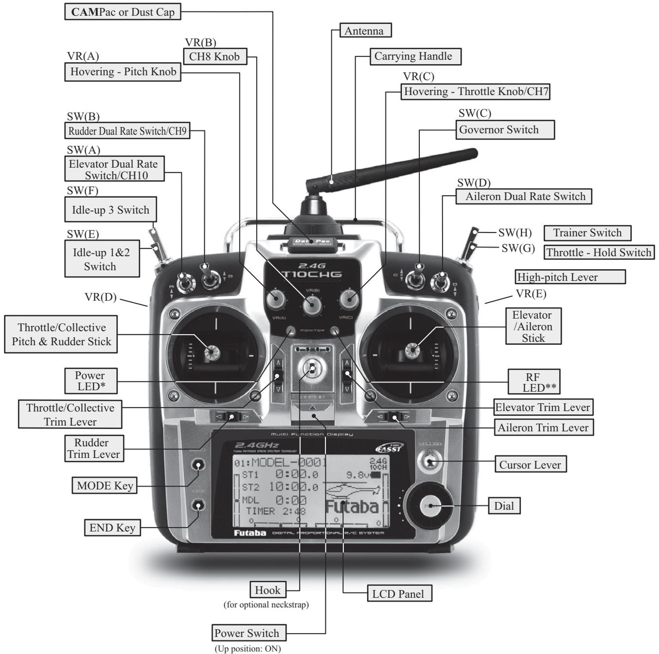
This figure shows the default switch assignments for a 10CHG Mode 2 system as supplied by the factory.
