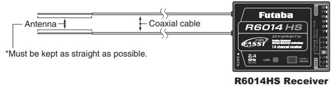
Futaba's dual antenna diversity then seamlessly selects the best signal reception between these antennas to ensure that there is no loss of signal.
