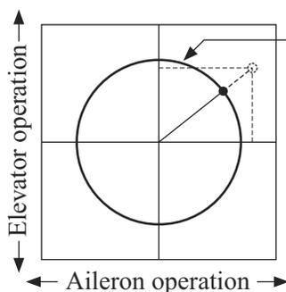
• Swash travel by simultaneous operation of the ailerons and elevators is limited within the circle (**SWASH RING** rate).
