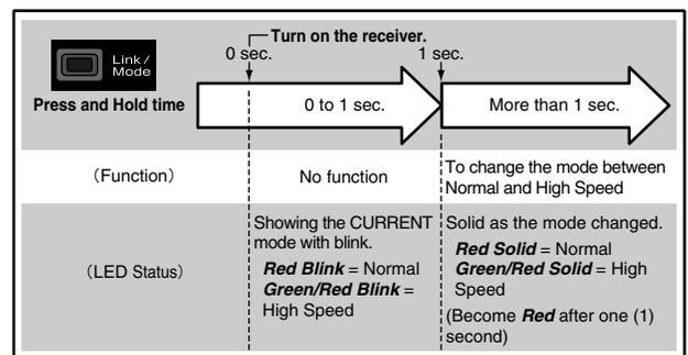
Please check the operation mode by observing the LED when turning on the receiver. If possible ensure that there's no FASST transmitter in operation near the receiver.
