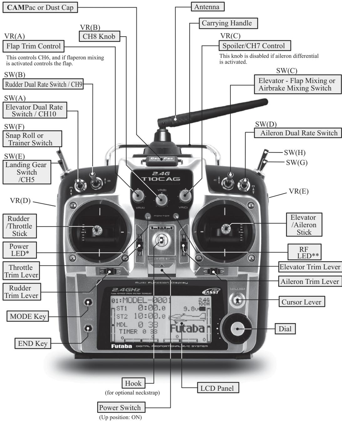
This figure shows the default switch assignments for a 10CAG Mode 2 system as supplied by the factory.
