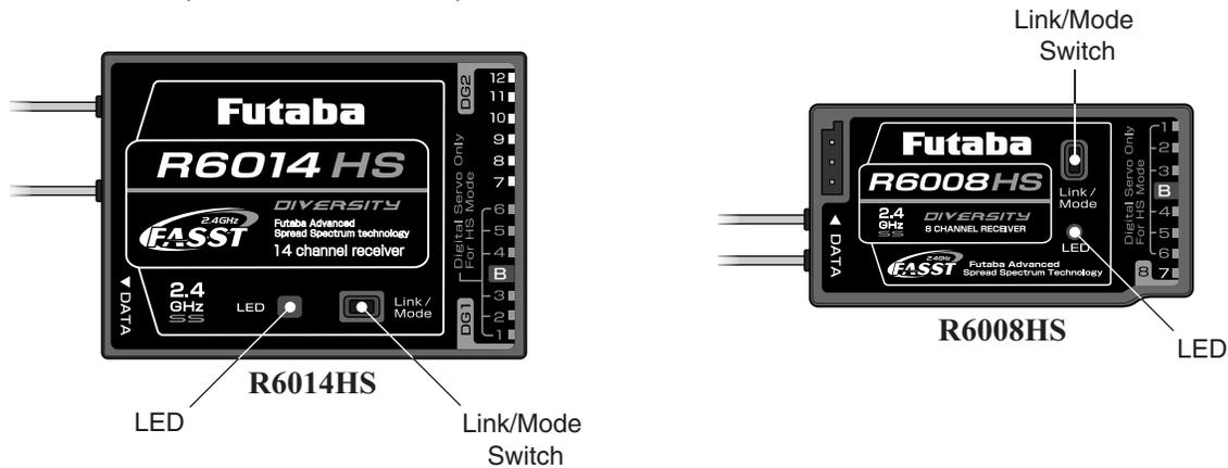
The operation mode is on "Normal mode" from factory shipping. To change the mode, please adhere to the following steps:
