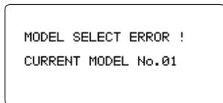
**Do not fly until the proper model is loaded into memory!** Reinsert the memory module, and recall the desired setup using the model select function.
