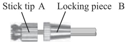
You may change the length of the control sticks to make your transmitter more comfortable to hold and operate. To lengthen or shorten your transmitter's sticks, first unlock the stick tip by holding locking piece B and turning stick tip A counterclockwise. Next, move the locking piece B up or down (to lengthen or shorten). When the length feels comfortable, lock the position by turning locking piece B counterclockwise.
