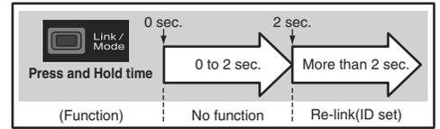
5. Press down the **Link/Mode** switch for more than two seconds, and release the switch. The receiver begins the linking operation.
