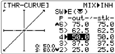
This function adjust the throttle operation curve for optimum engine response to throttle stick movement.
