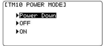
To activate the "Power Down Mode" press *DIAL* and the home screen will appear. During this mode, the RF power is reduced so the range test can be performed. In addition, when this mode is activated the blue LED on the front of the transmitter starts blinking and the transmitter gives users a warning with a beeping sound every 3 seconds.
