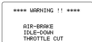
The **MIXER ALERT** warning is displayed to alert you whenever you turn on the transmitter with any of the mixing switches active. This warning will disappear when the offending switch or control is deactivated. Switches for which warnings will be issued at power-up are listed below:
