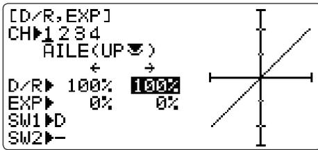
**Dual/Triple Rates:** reduce/increase the servo travel by flipping a switch, or (**ACRO/GLID**) they can be engaged by any stick position. Dual rates affect the control listed, such as aileron, not just a single (ex: channel 1) servo. For example, adjusting aileron dual rate will affect both aileron servos when using **FLAPERON** or **AIL-DIF**, and both aileron and elevator servos' travel when using **AILEVATOR** or **ELEVON** or a CCPM helicopter.
