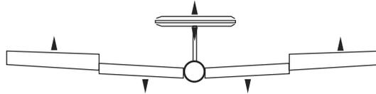
**BUTTERFLY** (often called "crow"- see **GLID**, p. 80 for details) simultaneously moves the flap, twin ailerons and elevator, and is usually used to make steep descents or to limit increases in airspeed in dives. Two separate **BUTTERFLY** settings are available. (**CIR1/CIR2**)
