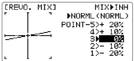
**REVO. MIX**: This 5-point curve mix adds opposite rudder input to counteract the changes in torque when the speed and collective pitch of the blades is changed.
