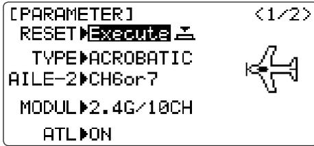
**AILE-2** only tells the radio that you are using CH5 and CH6 (**FLAPERON**), or CH5 and CH7 (**AILE-DIFF**), not CH6 or CH7, as the second servo in **FLAPERON** or **AILE-DIFF**. You still must activate and set up the **FLAPERON/AILE-DIFF** function.
